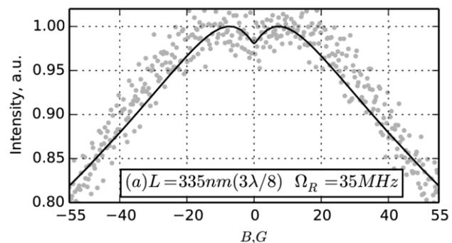
Fig.1 Magneto-optical resonance shape measured in ETC for Cs D<sub>1</sub> transition  $F_g=4 \rightarrow F_e=4$  at cell thickness of 335 nm (points – experiment, solid line – theory)
