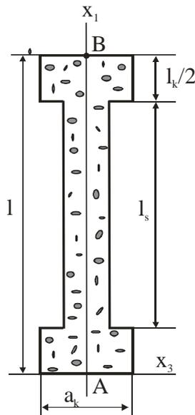
Fig.1. Platelet-shaped nanoparticles (in an increased scale) filling a polymer load-carrying element.
