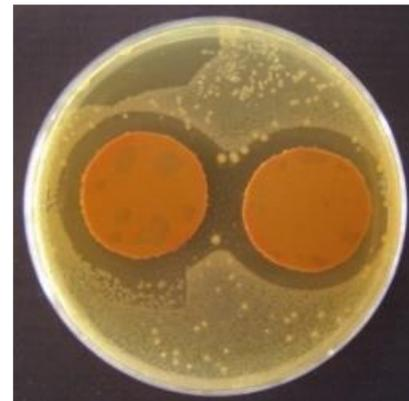
Fig.1 Antimicrobial activity of leather modified with Ag NPs.
