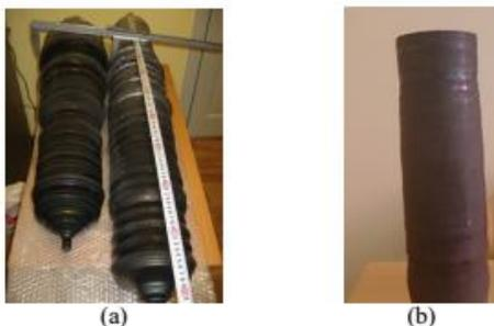
Fig.2 Rods grown without (a) and with (b) stabilization
