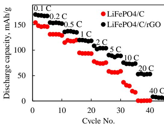
Fig.1 Rate capabilities of LiFePO<sub>4</sub>/C and LiFePO<sub>4</sub>/C/rGO composites
