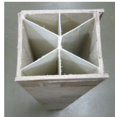
Fig.1. Example of plywood and GF/PP sandwich structure
