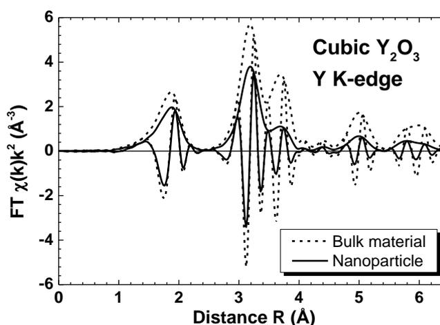
Fig. 1. Fourier transforms (modules and imaginary parts) of the calculated Y K-edge EXAFS for bulk material (dashed lines) and 1 nm nanoparticle (solid lines) cubic  $Y_2O_3$ .
