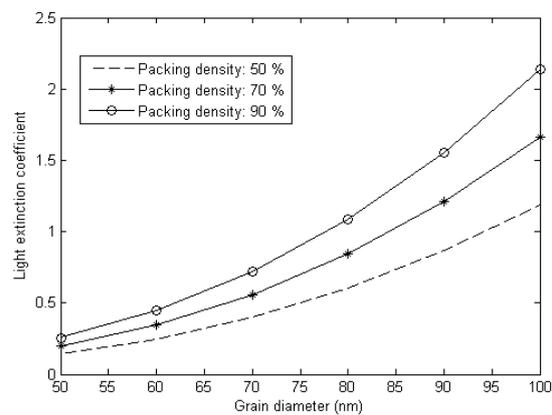
Figure 1: The variation of light extinction coefficient as a function of grain diameter (50 – 100 nm). Data are provided for three different values of packing density (50 %, 70% and 90 %).
