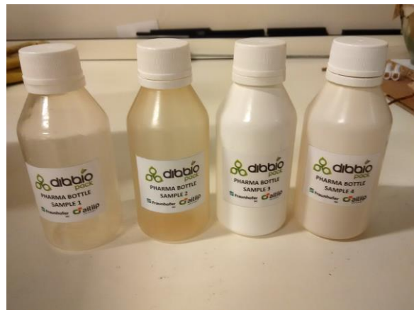
Fig.1 - Pharmaceutical bottle applications manufactured using Dibbiopack material formulations on Extrusion-Blow Moulding
