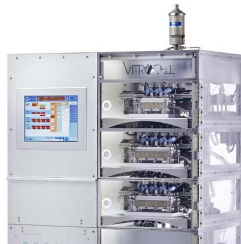
Fig.1 VITROCELL Automated Exposure Station equipped with 11 positions for the air-liquid interface exposure of cell cultures and one position for online particle dose determination.
